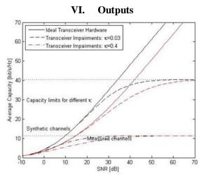
Fig 2 Average capacity of a 4x4 MIMO channel over different deterministic channel realizations, different levels of transceiver impairments, and  $\alpha = 1$  and k=0.03 and k=0.4
